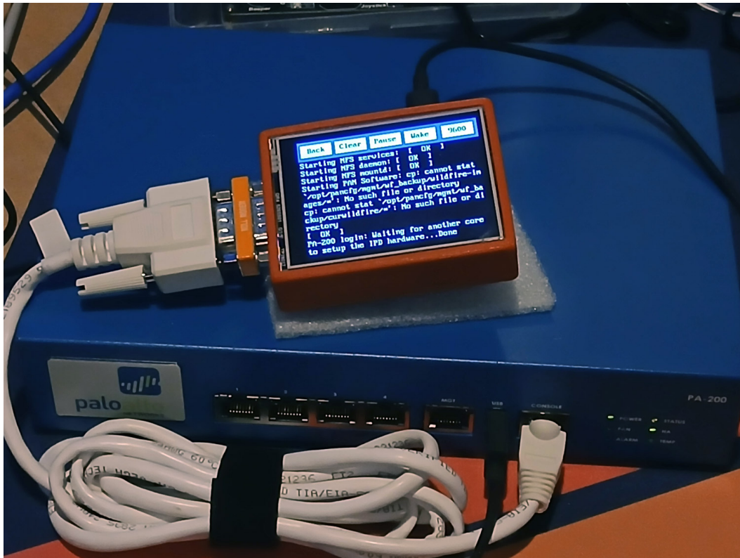
Figure 7.1: FortressFlash connected to a Palo Alto PA-200 firewall. The device successfully displayed the PA-200 console boot sequence using the same RJ-45 rollover cable and null-modem chain as with the FortiGate 60E, confirming cross-vendor compatibility at the console layer.
