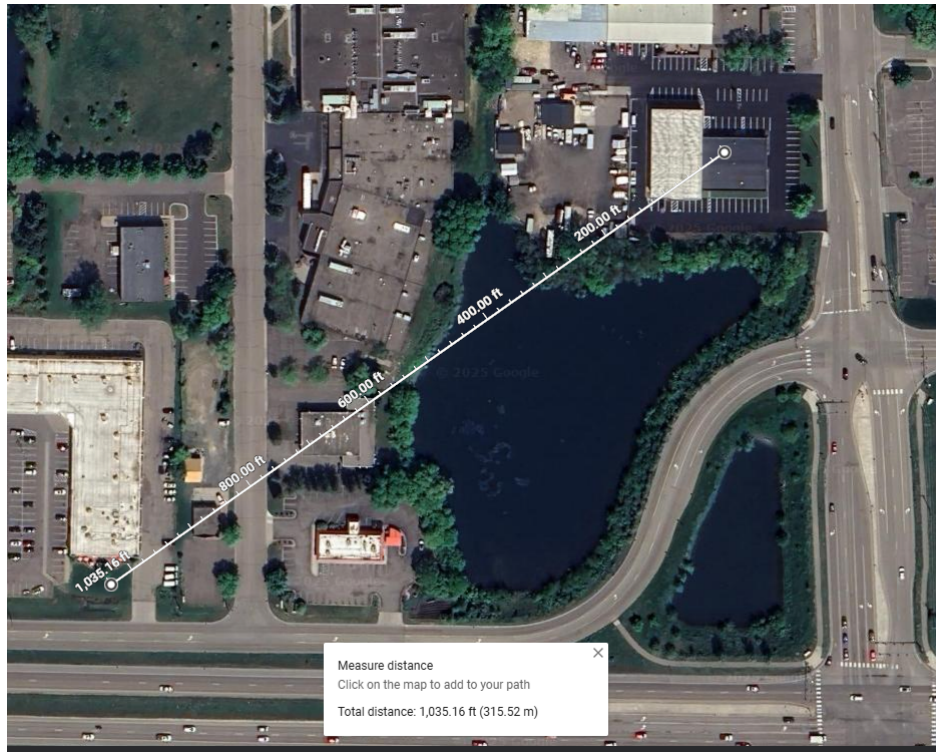
Figure 7.4: Google Maps screenshot showing the measured straight-line distance between the Fortress-Flash HQ base station and the farthest location where a successful auto-reply was received, totaling 315 meters (1,035 feet).
